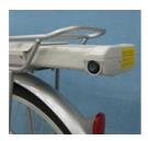
Battery can be removed from the case by unlocking the key lock
