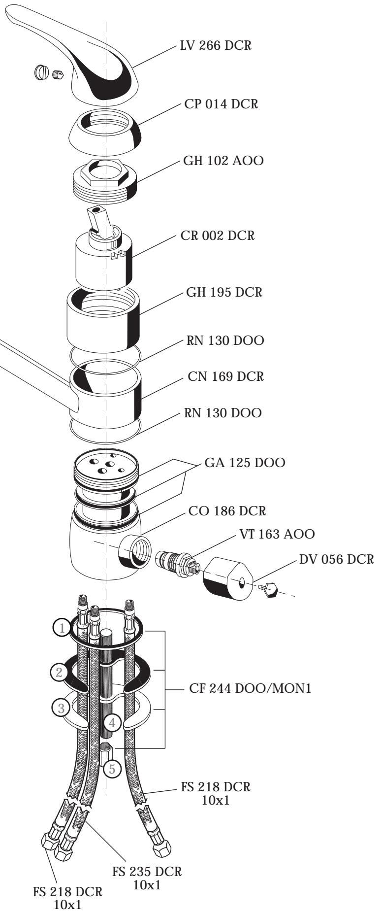
**(GB)** Screw the flexibles and lock screw 4 to the mixer body. Set down the rubber ring 1 in the groove placed at the bottom of the mixer body and then place the body on the sink or on the workplace. Push first rubber packing 2 and then the lockdisk 3 over lock screw 4 and tighten with nut 5.
