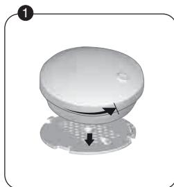
① Separate the 2 parts of the unit.
