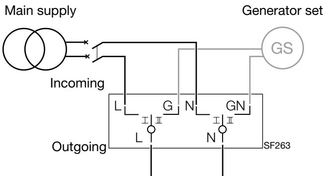
(EN) This modular changeover switch is not a disconnector. The isolation must be ensured with an appropriate device. The changeover incoming must be protected against short circuit with an appropriate MCB 63A - 4,5kA - Curve C.
